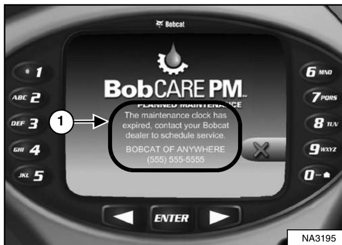
The Deluxe Instrumentation Panel will display a message (Item 1) [Figure 291] alerting the operator to service the machine.
