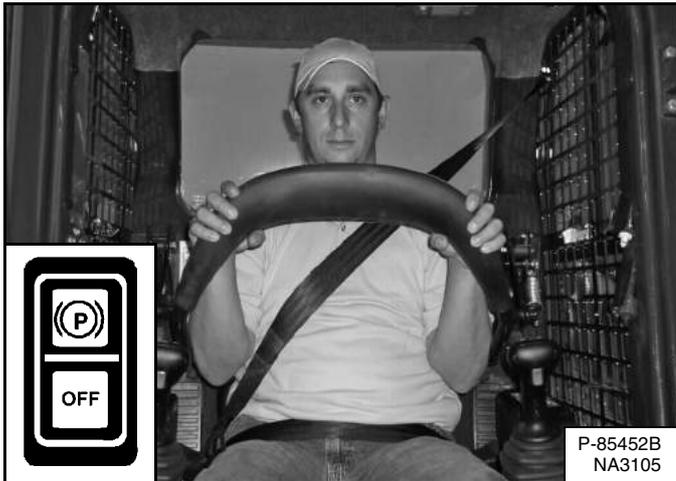
Lower the seat bar and engage the parking brake [Figure 126].
