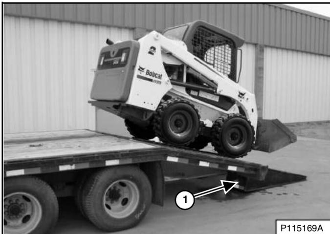
A loader with an empty bucket or no attachment must be loaded backward onto the transport vehicle [Figure 161].
