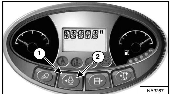
Press the button (Item 2) to engage auto idle. The light (Item 1) [Figure 56] is ON.
