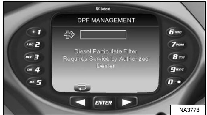
The machine will alert the operator when DPF service is required [Figure 254].
