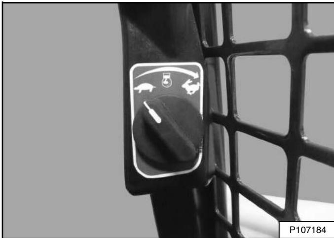
Set the engine speed control to the low idle position [Figure 128].
