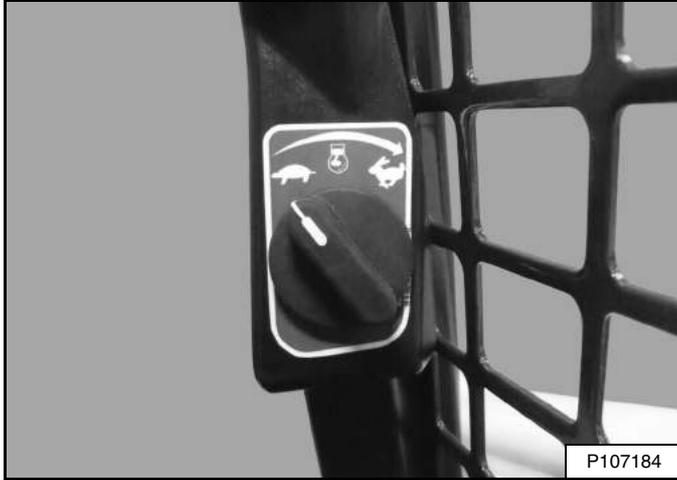
Set the engine speed control to the low idle position [Figure 134].
