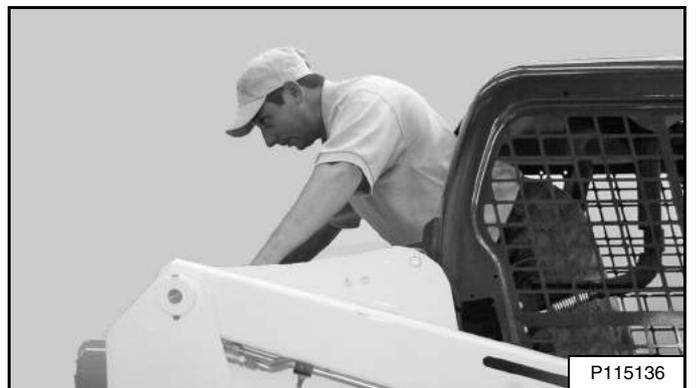
Exit through the rear of the operator cab [Figure 62].
