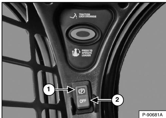
Press the top of the switch (Item 1) [Figure 52] to engage the parking brake. The red light in the switch will turn ON. The traction drive system is locked.
