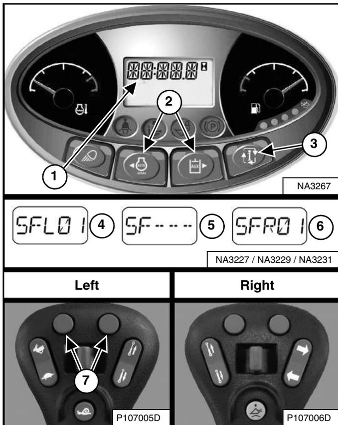
Press the Information button (Item 3) to cycle the data display until the steering drift compensation menu is displayed. The current steering drift compensation setting will appear in the data display (Item 1) [Figure 88].
