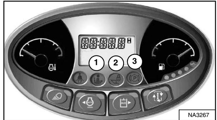
There are three display lights (Items 1, 2, and 3) [Figure 33] located on the left instrument panel that must be OFF to fully operate the machine.
