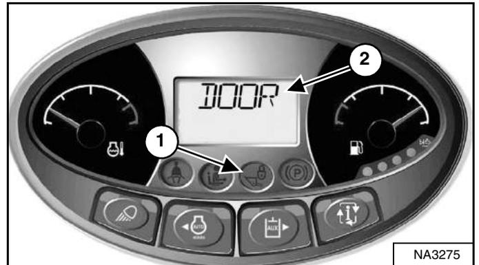
The LIFT AND TILT VALVE light (Item 1) [Figure 179] is OFF when the door is closed, the key switch is turned to RUN, the seat bar is lowered, and the PRESS TO OPERATE LOADER button is pressed.
