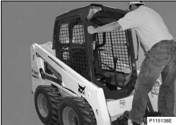
Use the bucket or attachment steps, grab handles, and safety treads (on the loader lift arms and frame) to get on and off the loader, maintaining a three-point contact at all times [Figure 118]. Do not jump.
