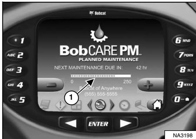
The Deluxe Instrumentation Panel will display a bar (Item 1) [Figure 292] showing the time remaining until next service. This bar will turn red when service is past due. [NEXT MAINTENANCE DUE] will change to [MAINTENANCE PAST DUE] and display the number of hours past due.
