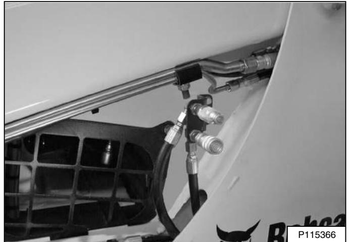
Move the Rear Auxiliary Hydraulic switch (Item 1) [Figure 106] or [Figure 107] to the right or left to change direction of the auxiliary hydraulic fluid flow to the rear quick couplers [Figure 108]. (Left side shown.) (EXAMPLE: Raise and lower rear stabilisers.) Release the switch to stop fluid flow.
