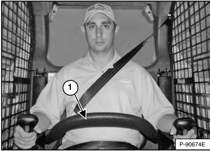
The Bobcat Interlock Control System (BICS™) has a pivoting seat bar with armrests (Item 1) [Figure 32]. The operator controls the use of the seat bar.
