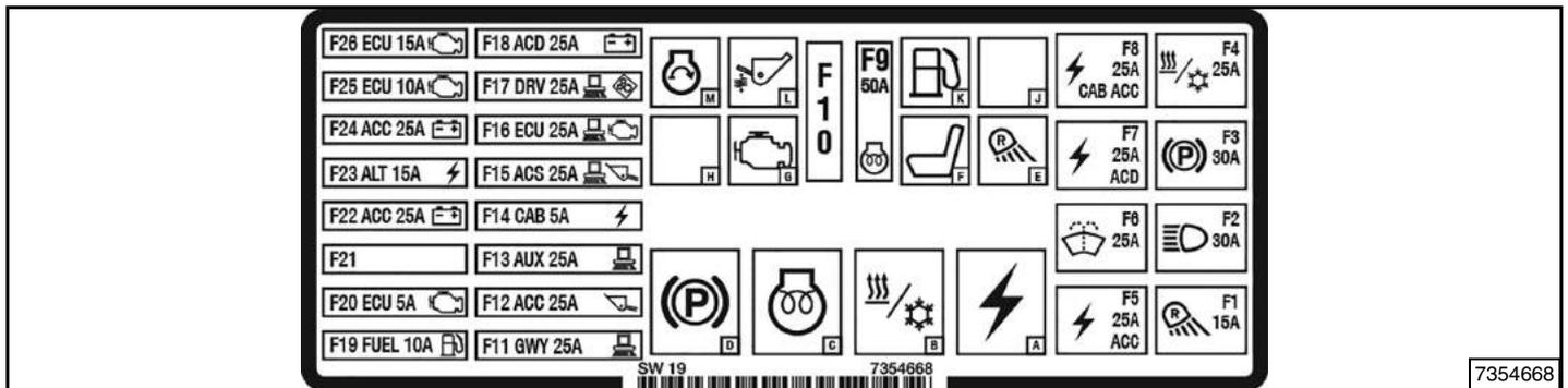
**SJC** - Fuse location and amperage ratings are shown in the table below and on the decal [Figure 236]. Relays are identified by the letter "R" in the AMP column.
