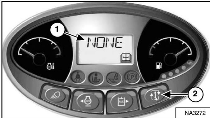
Press the Information button (Item 2) to cycle the data display (Item 1) [Figure 287] until the service code screen is displayed. If more than one service code is present, the codes will scroll on the data display.
