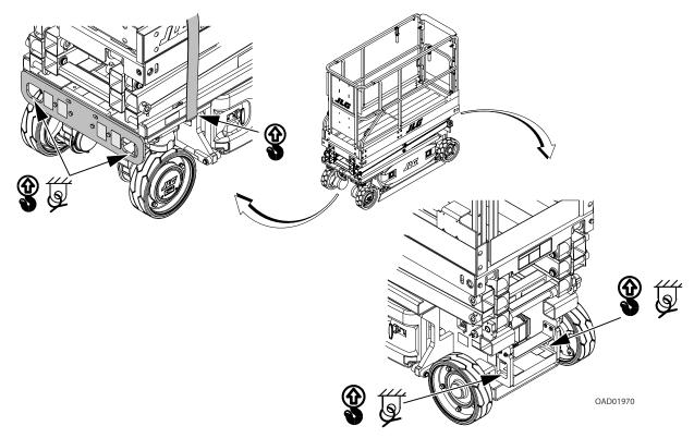
Figure 3-9. Lifting and Tie Down Diagram
