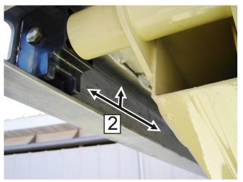
Figure 6-3. Upper Slide Pad Channel
