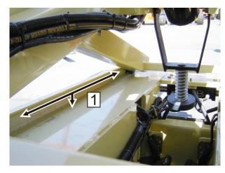
Figure 6-2. Lower Slide Pad Channel
