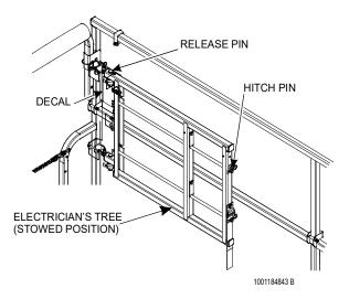
**NOTE:** The Electrician's Tree may be simultaneously installed with Panel Carrier, Pipe Racks, QuikWelder, or WorkStation as long as it in mounted on the opposite side of the platform.
