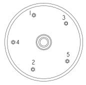
The tightening of the nuts should be done in stages. Following the recommended sequence, tighten nuts per wheel torque.
