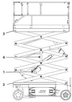
Figure 6-1. Lubrication Diagram
