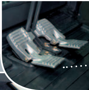
New ergonomic and foldable travel pedals improve cab comfort.
