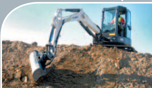
The tilt bucket is proportionally controlled by the joystick thumb switch.
