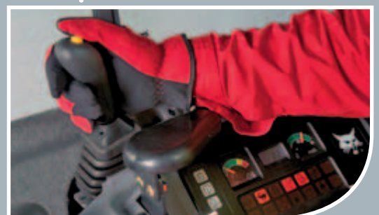
Third joystick controls blade flotation and second speed, for a more comfortable work environment.
