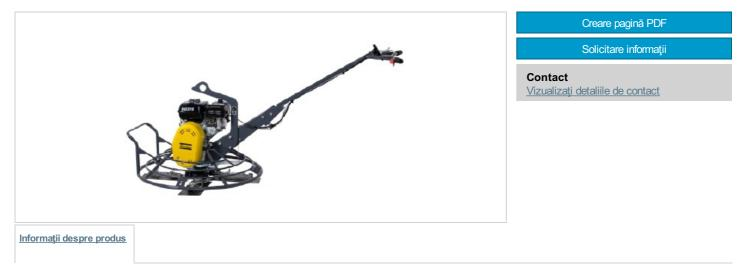
This high capacity trowels have 900 to 1,200 mm trowel diameters and power outputs from 5.5 to 9 hp. An adjustable handle with two different lengths makes work comfortable and safe.
